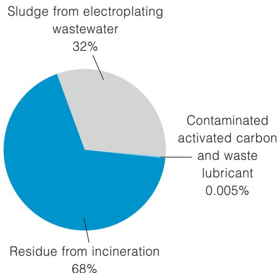
During the reporting year, the wastewater treatment facility at Eco-Plating Specialised Zone has been upgraded, not only to meet the tightened wastewater discharge standard set out by the Government, but also to significantly reduce the generation of hazardous sludge:
